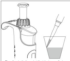
Place the pipette tip against the tube inner wall, at an angle of around 45°. Press the control button slowly to the first stop position and wait until the flow of liquid stops.
