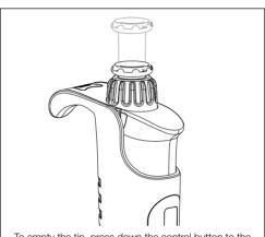
To empty the tip, press down the control button to the second stop. Hold down the control button and wipe the tip on the tube inner wall.
